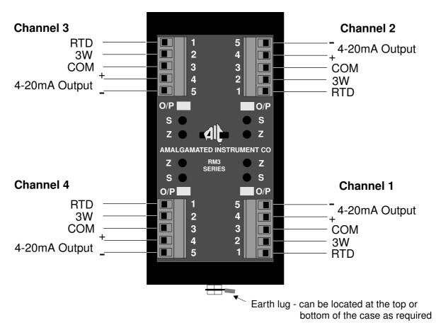
Data label example (located on instrument case)
