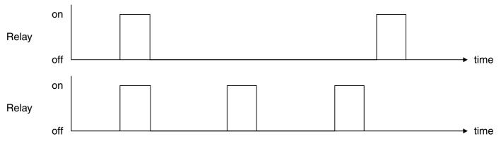
In frequency modulation mode the relay on time is fixed. A minimum relay off time can also be set. The control program will vary the actual off time to suit the error seen between the setpoint and the measured temperature at the time. For example if extra dosing is needed to reach the setpoint then the off time will be reduced resulting in more on pulses per period of time i.e. the frequency of the pulses is controlled to allow the setpoint to be maintained.
