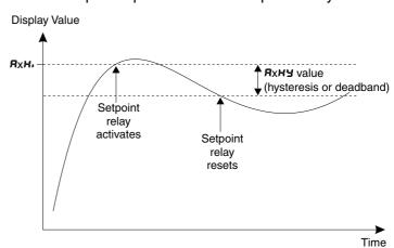
e.g. if **R IH**, is set to **50.0** and **R IHY** is set to **3.0** then the setpoint output relay will activate once the display value goes above **50.0** and will reset when the display value goes below **47.0** (50.0 minus 3.0).
