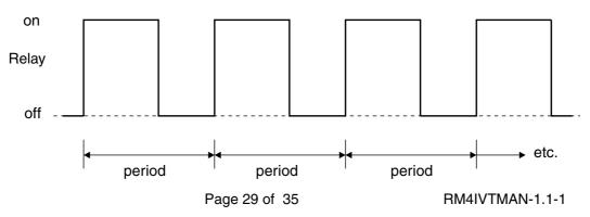
If set at 50.0 then the relay operation frequency will on for 50% and off for 50% of the duty cycle time when the measured input is at the setpoint. If set at 100.0 then the relay will activated for the whole time whist the measured input is at the setpoint.
