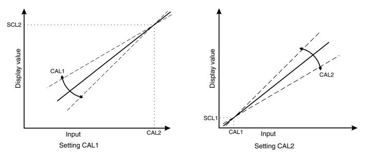
**CRL2** (second scaling point for 2 point scaling method).
