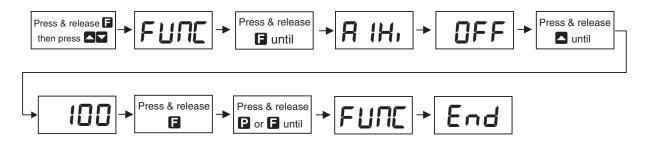
Example: Entering **ERL** mode to change decimal point function **deple** from **0** to **0.02**
