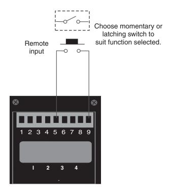
The selected remote input function can be operated via an external contact closure via a switch, relay or open collector transistor switch.
