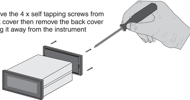
3. Remove the earth screw which passes through the underside of the case then slide out the board or boards
