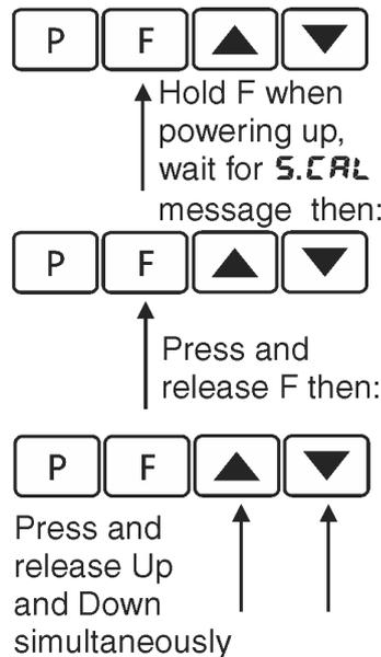
The setup functions are organised in blocks or sections e.g. all the settings for relay 1 are in the **RL 1** section. Once access to setup functions has been gained use the **▲** and **▼** buttons to select the section required then press **F** to enter this section and again use the **▲** and **▼** buttons to select the required function for alteration and press **F** to allow alteration of this function.
