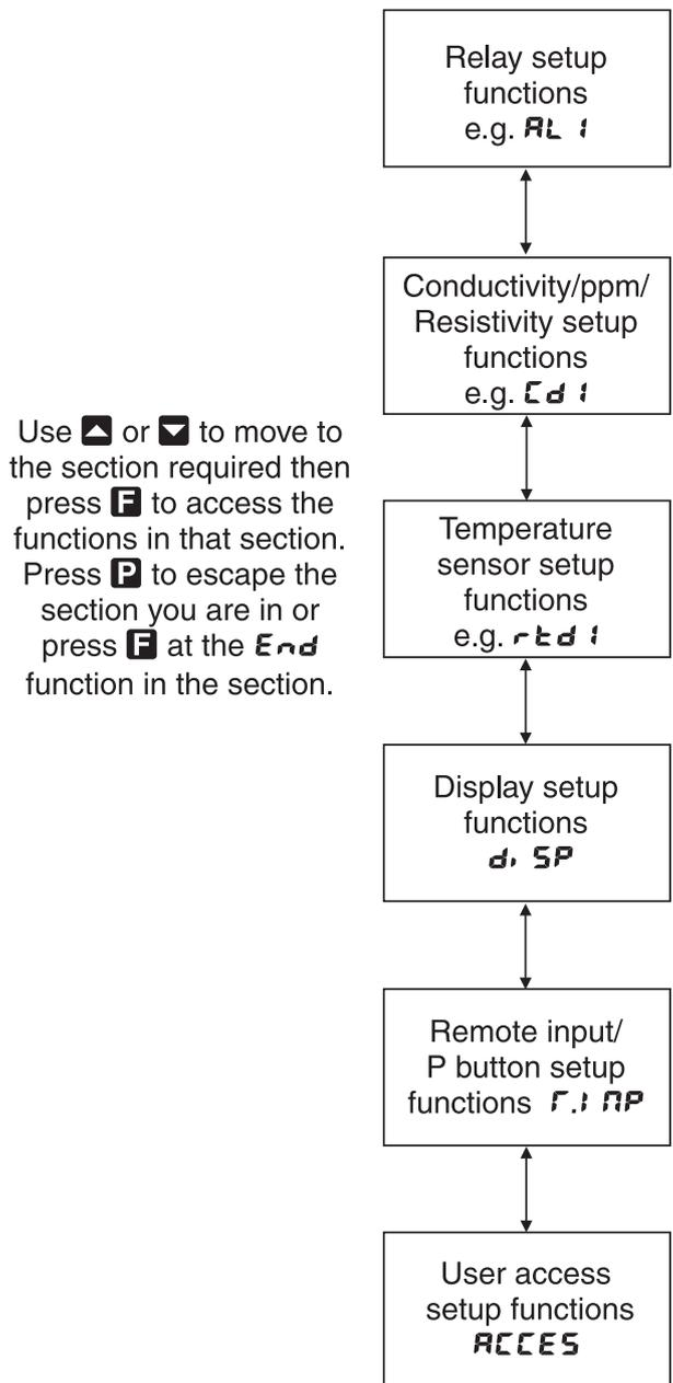
The example in the flowchart below shows the method using alarm relay 1 setup function.
