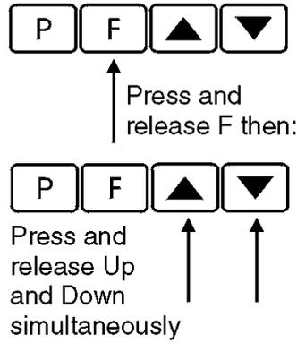
If a PIN has been set the message **Code** will be seen. Use **▲** or **▼** to enter the PIN then press **F** to accept the PIN.
