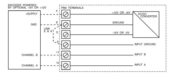
The optional supply can also be configured for 10V or 24V DC power supply and connected as shown below. It is necessary to link terminals D and 8 to couple the power supply and input grounds. The maximum current available is 20mA @ 24V and 40mA @10V.
