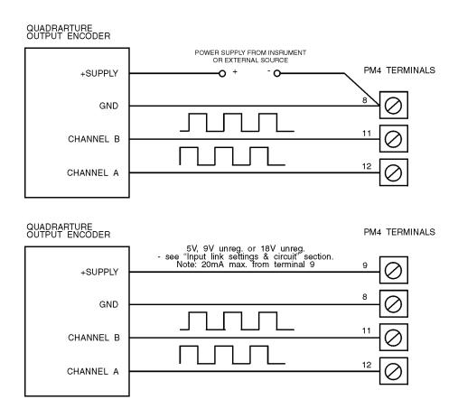
An optional 12V (or 5V) DC power supply is available and is connected as shown below. It is necessary to link terminals E and 8 to couple the power supply and input grounds. The maximum current available is  $40 \text{mA} \ @12V$  and  $80 \text{mA} \ @5V$ .
