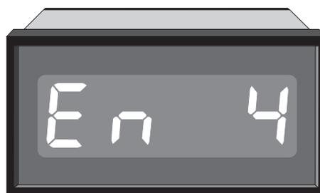
**▲** and **▼** buttons simultaneously. The display will now indicate **En 4** (enter 4 mA scaling value) followed by the last scaling value in memory. Using the **▲** or **▼** button set the display to the required reading for 4mA. Now press the **F** button. The display will indicate **En 20** (enter 20 mA scaling value) followed by the last scale value in memory. Now press the **▲** or **▼** button to obtain the required reading for 20 mA. Press **F** button the display will now
