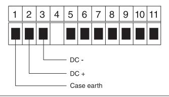
2 wire 4-20mA powered from non isolated regulated 18V supply (25mA maximum)
