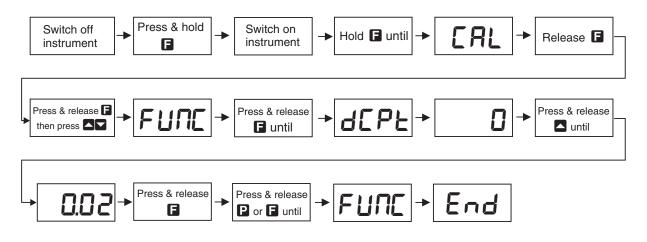
Easy alarm relay adjustment access facility
