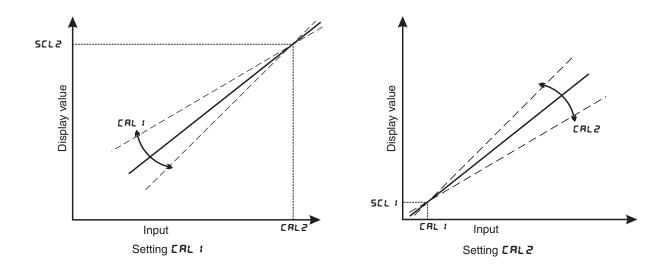
The procedure for entering the second scaling point **CRL2** is as follows:
