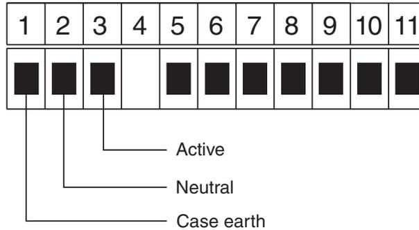
DC power connections (12 to 48VDC) - supply type is factory configured, check before connecting
