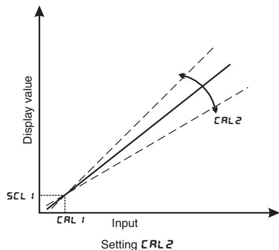
The procedure for entering the second scaling point **CAL2** is as follows:
