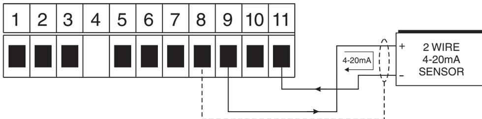
2 wire 4-20mA externally powered sensor
