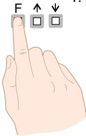
1. Remove power from the instrument and wait 5 seconds . Hold in the **F** button and reapply power. The display will indicate **CAL** as part of the "wake up messages" when the **CAL** message is seen you can release the button. Move to step 2 below.
