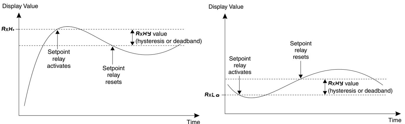
e.g. if **A 1H** is set to **50.0** and **A 1HY** is set to **3.0** then the setpoint output relay will activate once the display value goes above **50.0** and will reset when the display value goes below **47.0** (50.0 minus 3.0).
