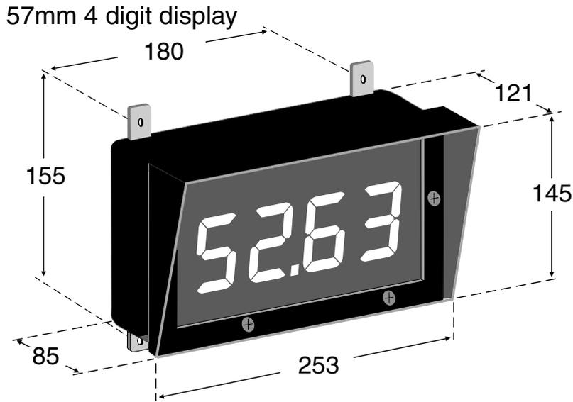
An optional panel mount kit is available for the 57mm type display. Panel cut out size is 240 x 130mm (-0.0mm/+0.5mm)
