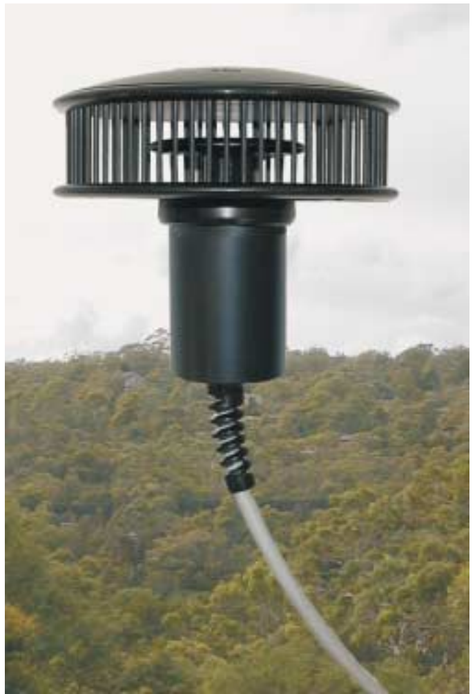
WS-MMW-005 shown clipped into orientation mount. Mount is bolted to a flat surface
