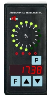
Circular graph and 5 digit display
