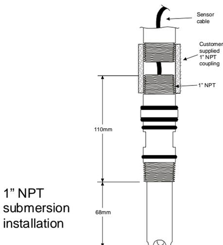
1" NPT submersion installation
