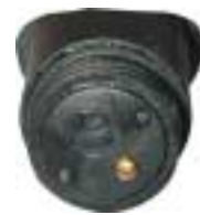
Detail of pH electrode tip showing the flat surface membrane, temperature sensor & reference junctions
