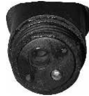
Detail of pH electrode tip showing the flat surface membrane, temperature sensors & reference junctions
