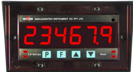
6 digit 38mm high LED (visibility to 18m)
