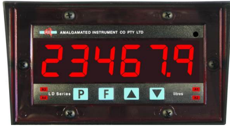
6 digit 38mm high LED (visibility to 18m)
