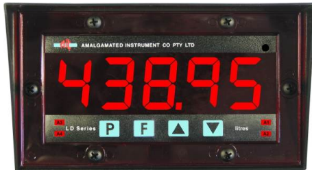
5 digit 45mm high LED (visibility to 20m)
