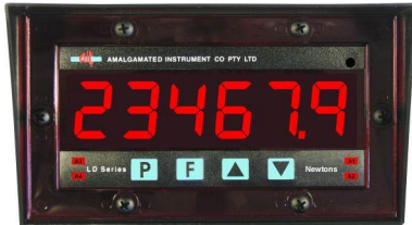
6 digit 38mm high LED (visibility to 18m)
